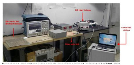
Nanosecond, high voltage pulse generation system designed and realized at IREA
