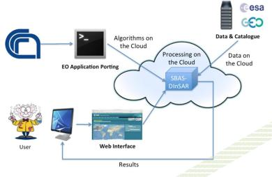
Schematic sketch of interferometric SAR processing in a cloud environment
