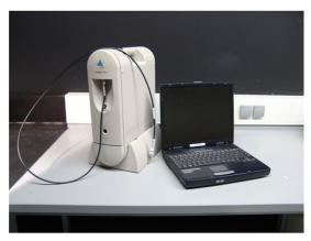
Portable spectroradiometer for field measurements (350-2500 nm spectral range)
