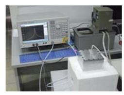
Microwave sensor for water pollutant detection developed at IREA
