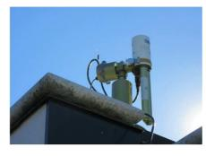
A photometer of the 'AERONET' network, positioned at the Archaeological site of Grotte di Catullo in Sirmione on Lake Garda, was inaugurated last October 22. The sun photometer Cimel is a tool that helps to measure the values of the optical thickness of the atmosphere and, therefore, it can be an interesting device to evaluate some c characteristics of the suspended particles in the atmosphere, such as their quantity and origin,
