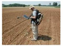
Measuring soil reflectance over agricultural land with a field spectroradiometer
