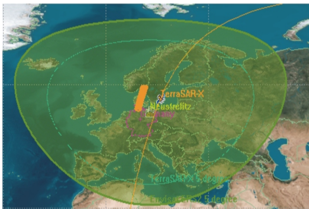
Figure 1: Ground Station Neustrelitz, acquisition circle for ERS2 and TerraSAR-X; 5 degree elevation
